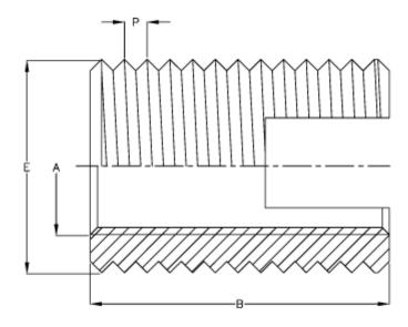
Female thread A = M12 Length B = 22 Male thread E = 16.0 Min hole depth blind hole = 26
